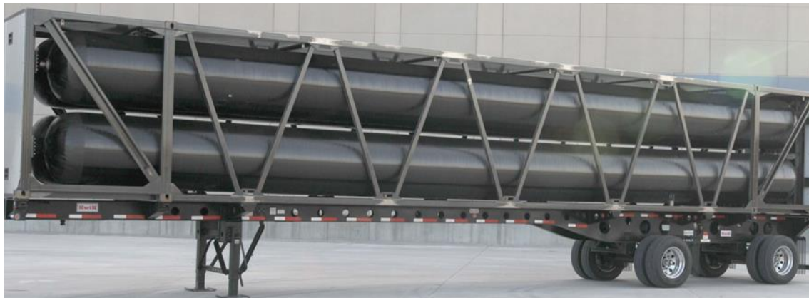
Figure 4-3: Four Maximus tanks by Hexagon Purus in a 40' trailer. Source: Hexagon
